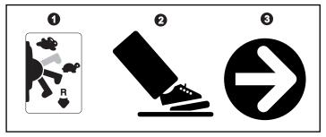
Please Note: To avoid damaging the motors and gears, stop the vehicle before shifting between low and high speed.
